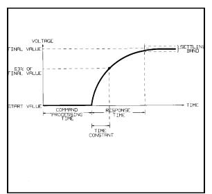
Figure 1-3. Output Response Characteristics
